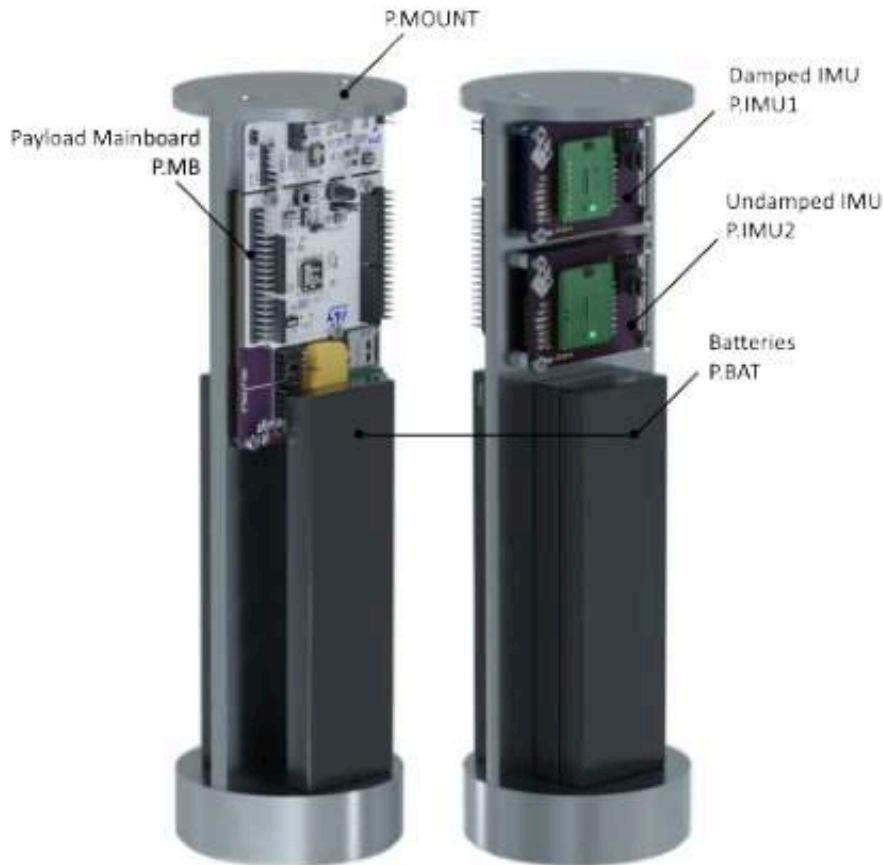
Fig. 43. Render of Payload with components marked.
