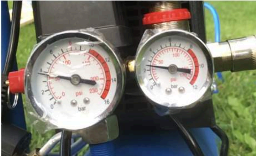
Fig 30: Shear pressure: measured at 2.5 bar, consistent shear for all screws.
