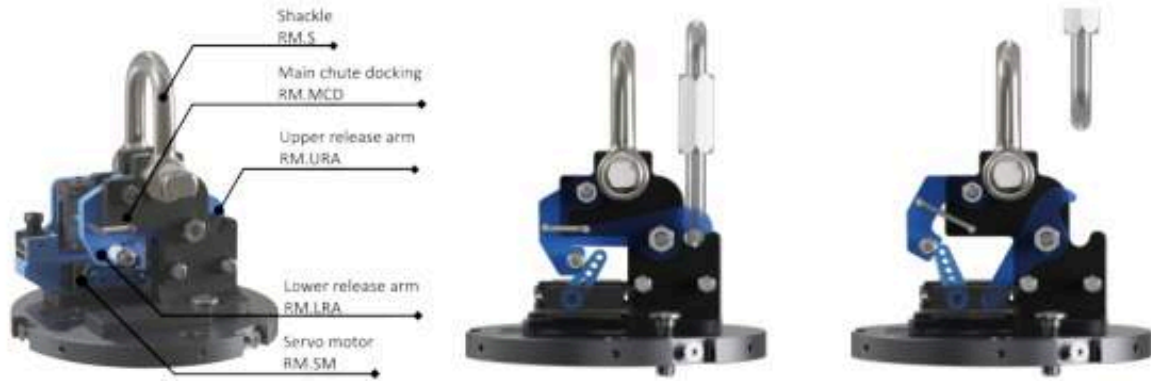
Fig. 33. MCRS overview (left), MCRS locked position (middle) and MCRS open position (right). Note that one of the two servos are hidden to display the mechanism more clearly.
