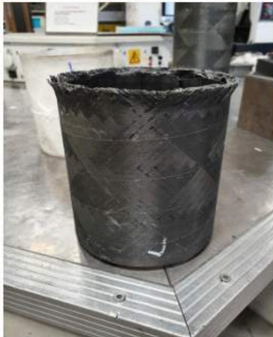
Fig 37: Carbon fiber section after test 3
