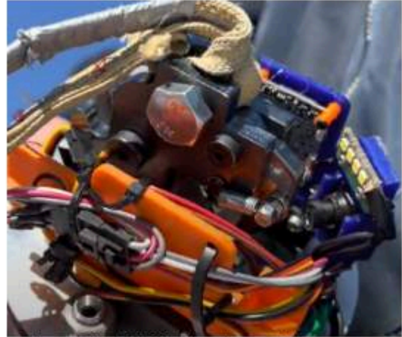
Figure 21: MCRS before launch. The springs are clearly not pretensioned
