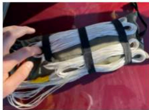
Fig 16: Parachute packed, shroud lines z-folded
