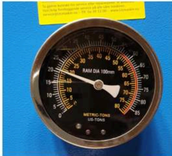
Fig 35: Force exerted on the test article when it yielded
