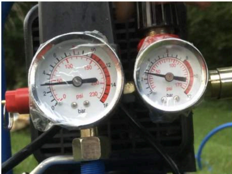
Fig 32: Shear pressure: measured at 2.7 bar, consistent shear for all screws.
