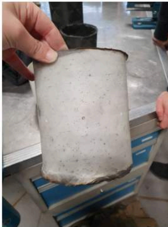
Fig 38: Fiberglass section with holes after test 4
