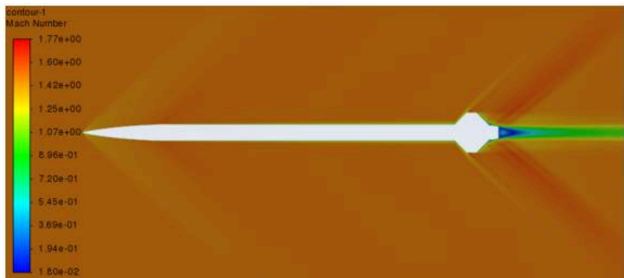
Figure 7: Contour plot of Mach numbers around the rocket at Mach 1.5
