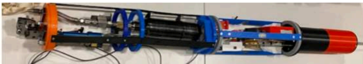
Fig 54: The Recovery, Avionics and Payload assembled
