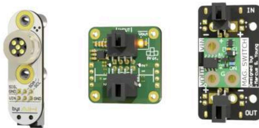
Fig. 38. From left to right, Mag. plug PCB, Circuit protection PCB and Mag. switch PCB.
